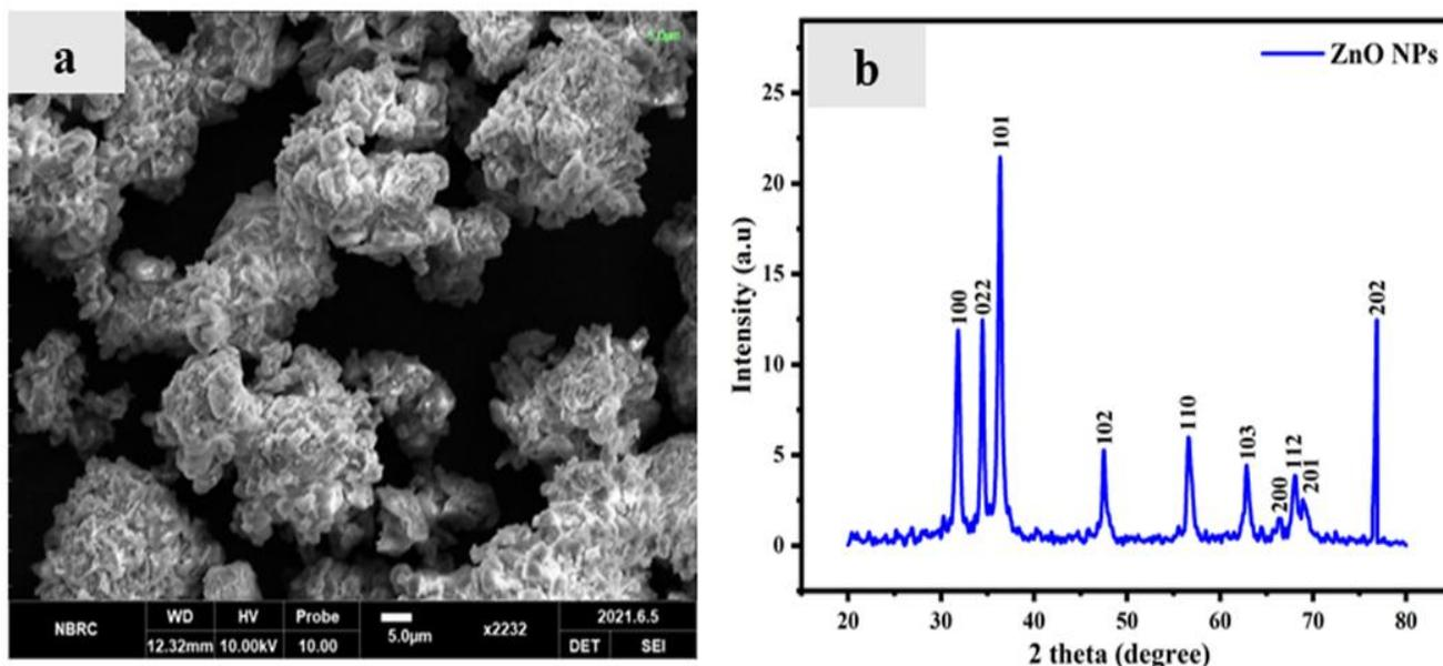
**Figure-1:** (a) The image of SEM exhibits of morphology of ZnO NPs (b) XRD shows structural properties of ZnO NPs.
